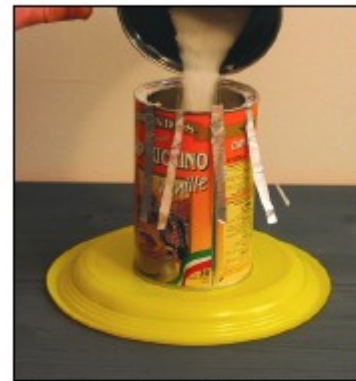
Making sweet, static electricity: (above) charging with sugar and discharging; the equipment (bottom).
